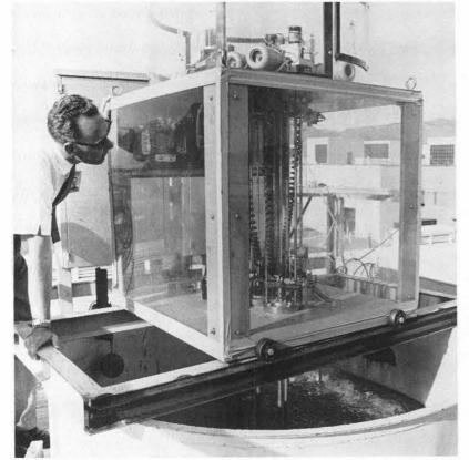
THIS CONTROL MECHANISM, being examined by F. A. Hasenkamp, is at the top of the 30 ft. high mock-up of the reactor core, and will eventually be moved to Area V. Core is water-cooled.
